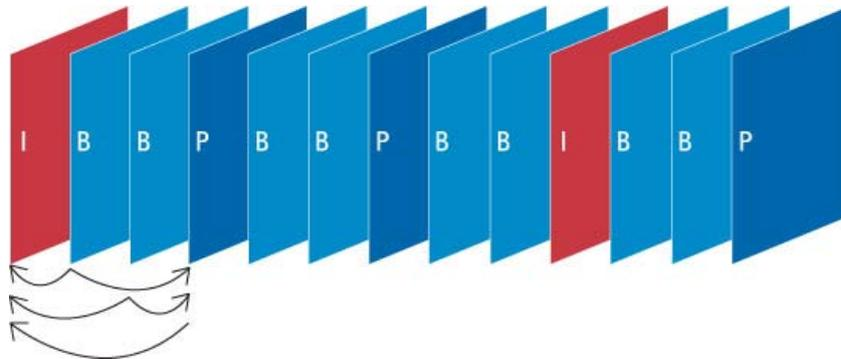
**Figure 5.** The illustration above shows how a typical sequence with I-, B-, and P-frames may look. Note that a P-frame may only reference a preceding I- or P-frame, while a B-frame may reference both preceding and succeeding I- and P-frames.
