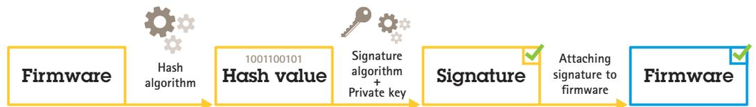
Figure 1. The process of signing firmware.
