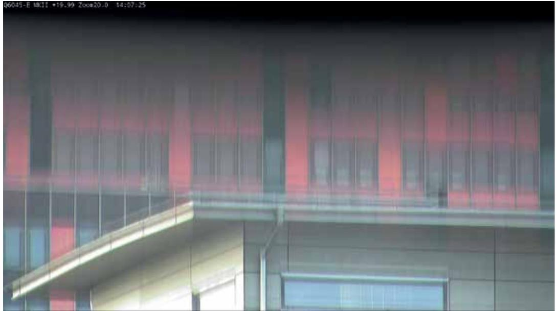
Figure 2: Mirroring in a conventional dome camera at 20° tilt, 20× zoom.
