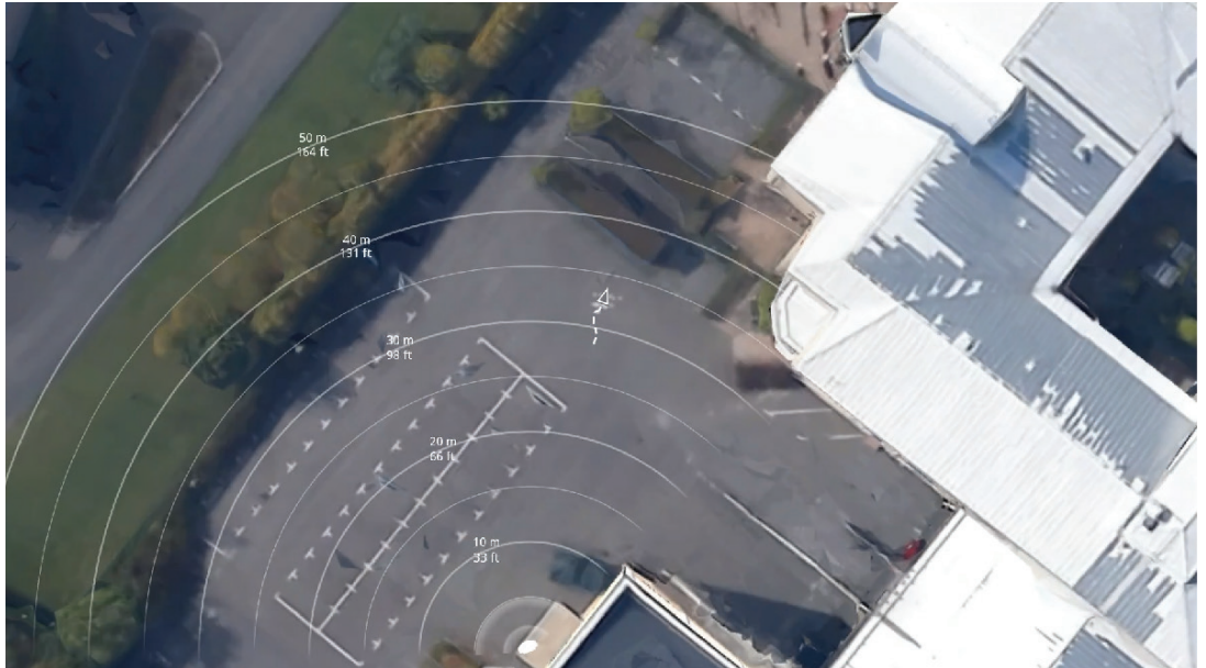
Figure 2. A scene (from above) monitored with AXIS D2050-VE Network Radar Detector, as showed in the user interface when combined with a reference map. The detector is mounted on the building at the bottom of the picture. The arrow just above the center of the image marks an object being tracked by the detector.
