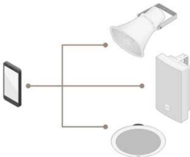
There are third-party SIP apps that can be used for making announcements to Axis speakers. Most manufacturers of telephony and unified communications equipment also have their own apps for smartphones. If these apps are supporting the SIP protocol, they may also be compatible with Axis IP speakers. Axis does not test the compatibility of such apps so it would be up to you or your integrator to do that.
