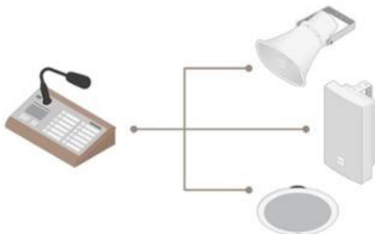
Public address (PA) systems enable the broadcasting of announcements in locations such as stadiums, schools, and shopping malls. Modern IP-based PA systems consist of IP audio devices, typically microphones and speakers, and audio management software which may be integrated in the devices. Announcements can be made live, played back according to a schedule, or triggered in response to specific events.
