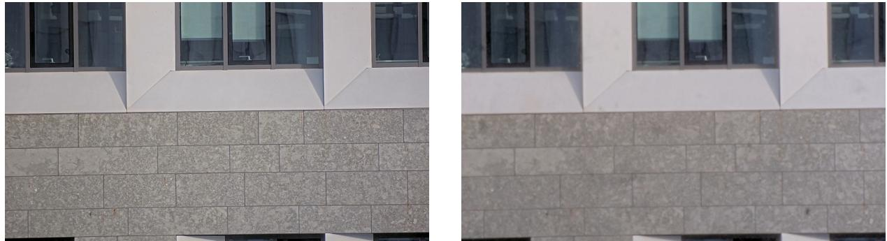
*An iris with a too small opening will cause diffraction, as seen in the image to the right.*
