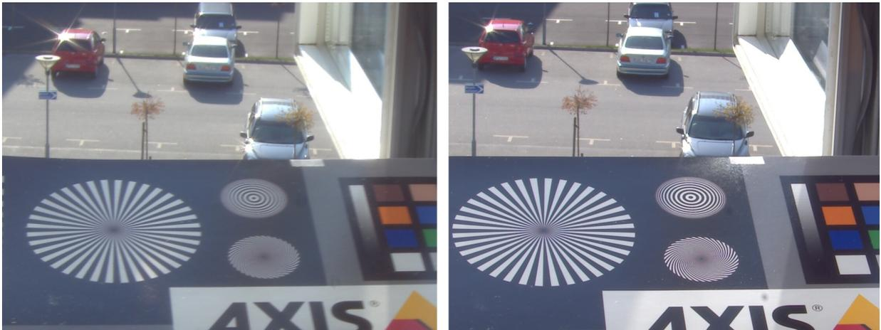
*The picture to the left was taken with a camera using a DC-iris lens. The picture to the right was taken with a camera using a P-Iris lens and exhibits sharper contrast than the picture to the left.*
