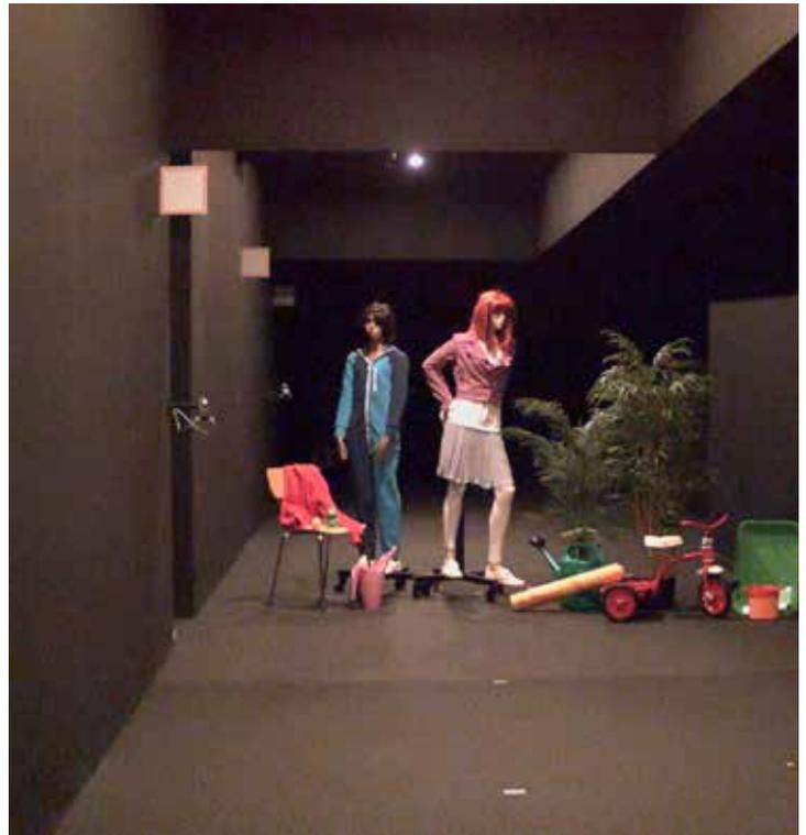
*Figure 6: 0.1 lux – 0.3 lux measured on the objects. The Lightfinder camera provides a less sharp, but still very detailed, image with colors. The human eye could not discern the darker surfaces and perceived no details or colors.*
