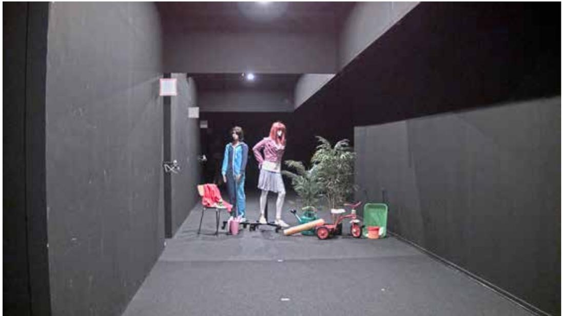
*Figure 4: A studio scene with a light intensity between 1.5 lux (on the tricycle) and 5 lux (at the mannequins' waists). The Lightfinder camera delivered clear colors and a deceptively bright image, while a human eye could also discern color but perceived the scene to be very dark.*
