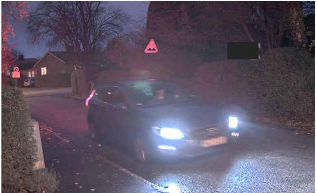
*Figure 8: A long exposure time may cause visible motion blur. In this video snapshot, the license plate could have been readable if a shorter exposure time had been used.*
