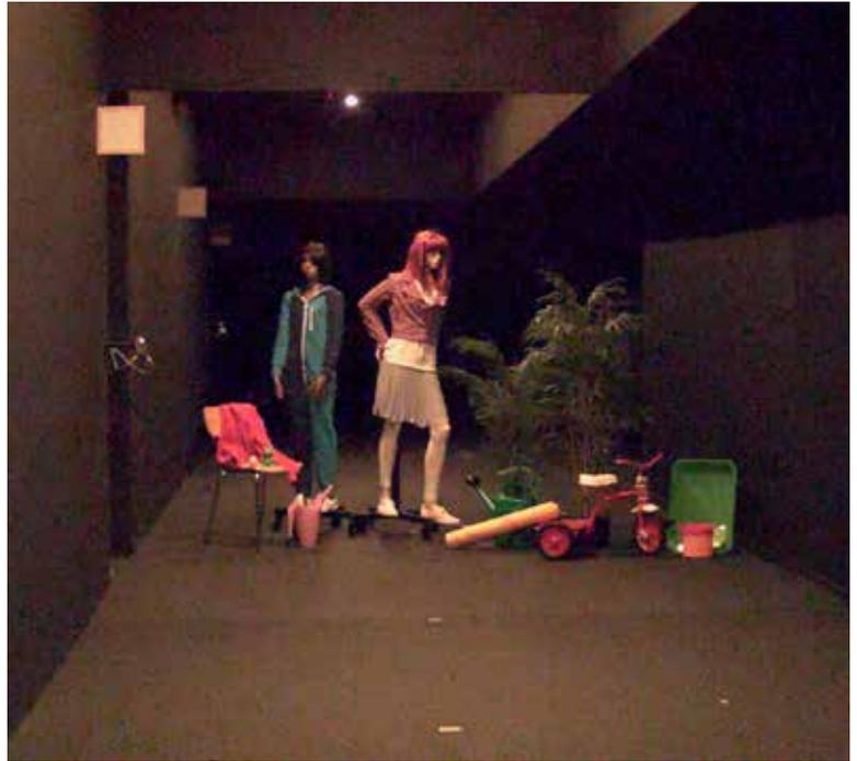
*Figure 7: 0.02 lux – 0.08 lux measured on the objects. The Lightfinder camera provides a dark image with subdued but discernible colors. The human eye could only vaguely discern the lightest surfaces and perceived no details or colors whatsoever.*
