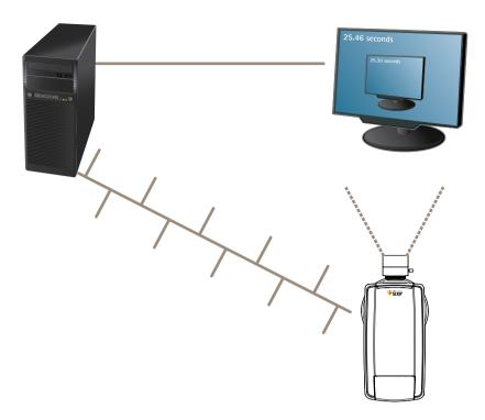
From the picture above you can see the time difference is 460 ms - 300 ms which gives us an end-to-end latency at 160 ms.
