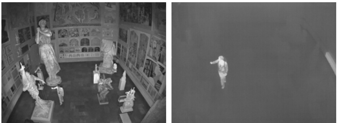
Figure 4 and 5: To the left an image from a day-and-night camera with integrated IR illumination, and to the right an image from a thermal camera, passively detecting heat radiation.
