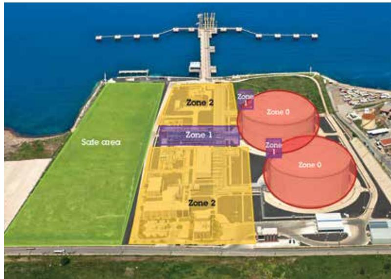
Figure 14. An industry facility with areas classified into different Zones.
