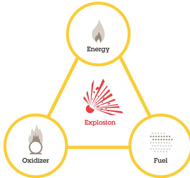
Figure 2. The three components that must be present for an explosion to occur.
