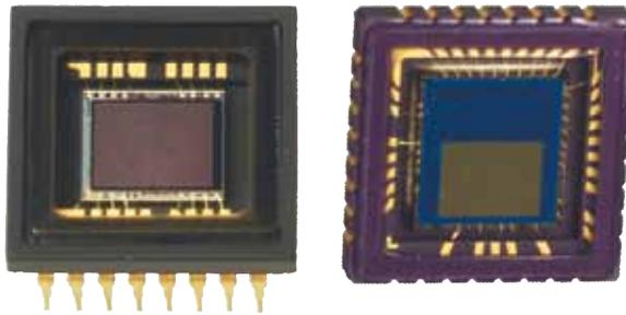
Figure 1. Image sensors: CCD (left) and CMOS (right)
