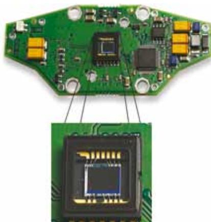
Figure 4. CCD sensor mounted on a PCB
