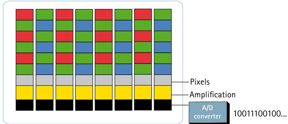
Figure 5. CMOS sensor
