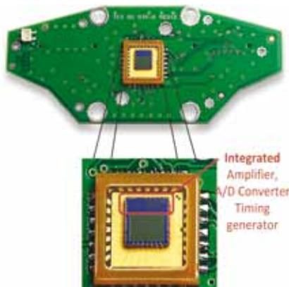
Figure 6. CMOS sensor mounted on a PCB
