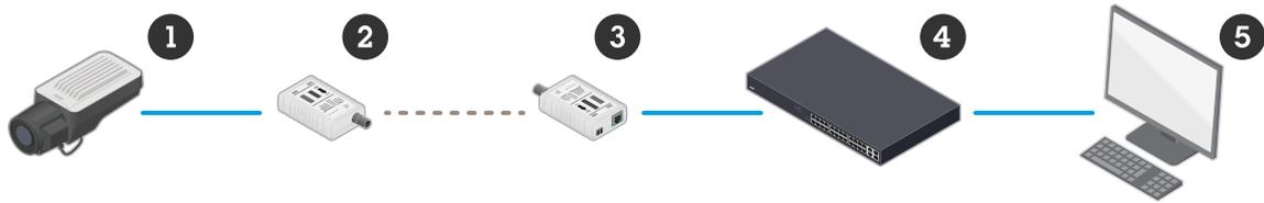
Figure 9. A network video system that utilizes a PoE+ over coax adapter kit (device adapter (2) and base adapter (3)) to combine IP cameras (1) and existing coax cabling. The system is connected to the network and to a VMS using a network switch (4) and a computer (5).
