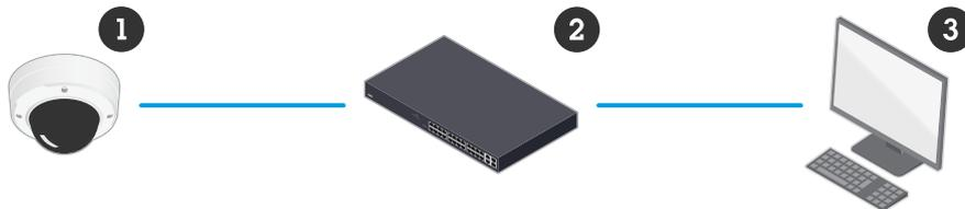
*Figure 11. A true network video system where video from network cameras (1) is continuously transported over an IP network. This system takes full advantage of digital technology and provides consistent image quality from the cameras to the viewer at whatever location, enabled by a PoE switch (2) and a computer with a VMS (3).*
