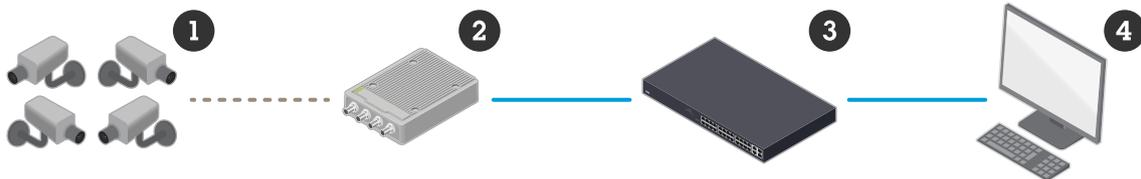
*Figure 1. Analog cameras (1) can use legacy coaxial cabling to connect with a video encoder (2). The video encoder digitizes the video and sends it over LAN to a network switch (3) which can pass it on to video management software (VMS) (4).*
