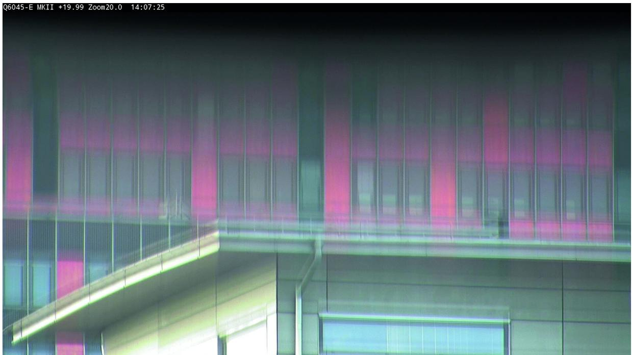
Figure 1. Mirroring in a conventional dome camera at 20° tilt, 20× zoom.
