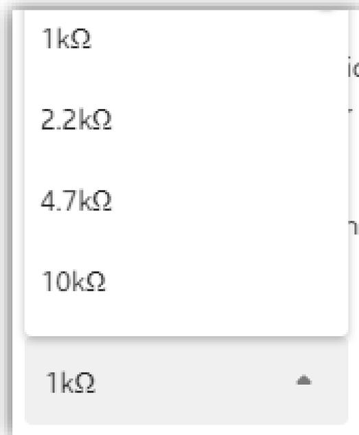
Under **Door monitor**, **Emergency input**, **Wiegand tamper** and **REX** there is a possibility to configure a input supervision, meaning the possibility to detect tampering attempts on the cable by measuring a specific connection with end of line resistors mounted as close to the peripheral device as possible.
