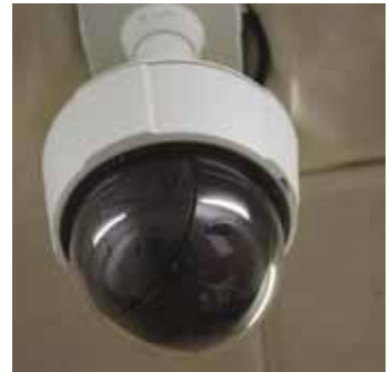
AXIS P5534 PTZ photographs and sends an image of the monitor after receiving an alarm signal.
