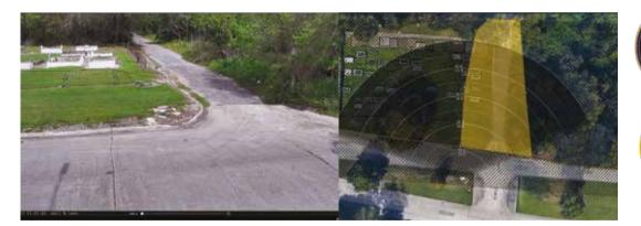
When the Axis network radar detector senses an event, it redirects the PTZ camera from its default position to track and record culprits illegally dumping.
