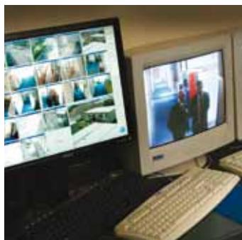
Two AXIS 241Q Video Servers with four analogue cameras on each are deployed to take images from existing analogue cameras and relay them into the network. A total of 18 AXIS 211 Power-over-Ethernet Network Cameras, and one AXIS 2130 PTZ Network Camera were deployed across the entire campus. A total of 27 cameras feed into the Milestone XProtect® Enterprise Version 5.0 system for handling, storage and management of camera output.
