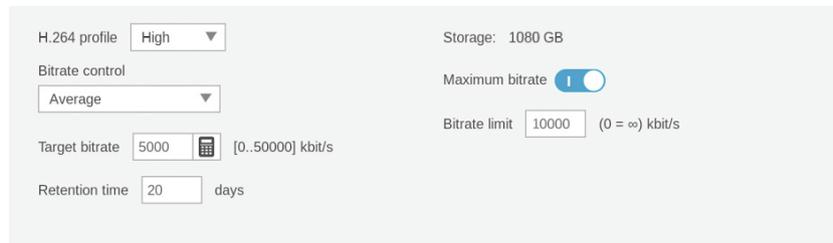
The image shows a configuration panel for a camera's ABR settings. It includes a dropdown for 'H.264 profile' set to 'High', a 'Storage' indicator at '1080 GB', a 'Bitrate control' dropdown set to 'Average', a 'Maximum bitrate' toggle switch that is turned on, a 'Target bitrate' input field with '5000' and a calculator icon, a 'Retention time' input field with '20' and 'days', and a 'Bitrate limit' input field with '10000' and '(0 = ∞) kbit/s'.
