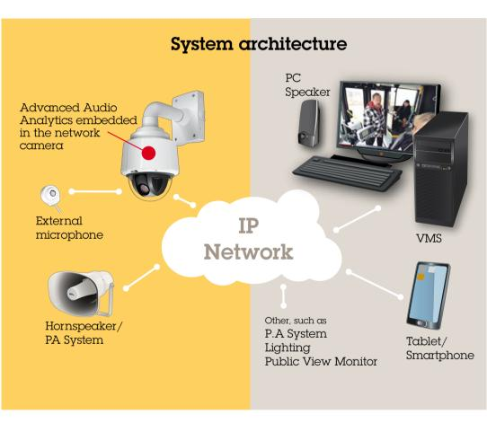
When embedded audio analytics detects sound patterns for characteristics of aggression, glass break or gun shots, the system will trigger the camera to stream real-time video footage to a control room or mobile device.
