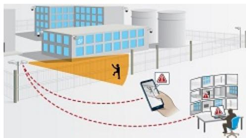
Combined with network cameras, network horn speakers and video management software, AXIS Perimeter Defender forms a comprehensive, video-based solution for effective perimeter surveillance and protection.
