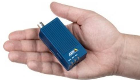
The video encoder is suitable for all analog camera types, both fixed and pan/tilt/zoom cameras. Featuring Power over Ethernet (PoE), the same Ethernet cable is used for both data and power, making installation flexible and easy. The video encoder also features a card slot for edge storage with microSD cards or NAS (Network-Attached Storage). AXIS Camera Companion and AXIS Video Hosting System are supported.
