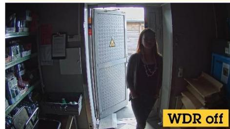
*Axis Forensic WDR technology enable surveillance operators to see forensic levels of detail in scenes with both bright and dark areas, even in surveillance areas with high levels of motion or when using ultra-high resolution cameras. Above image shows how it can look with or without Forensic WDR.*
