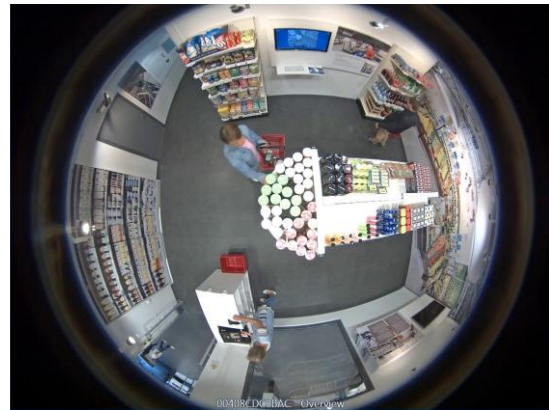
AXIS Camera Companion 2.1 includes de-warping which converts the 360° view to a traditional format for investigation of details.
