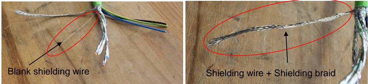
Figure 2.3 – Blank shielding wire and shielding braid
