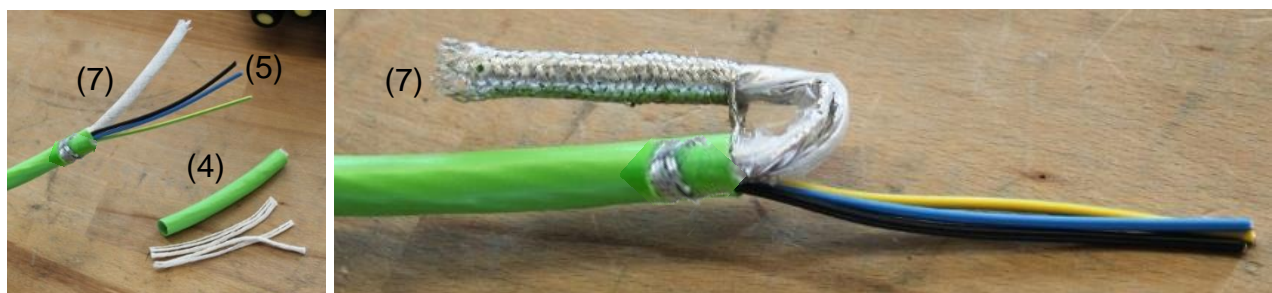
Figure 2.2 – Stripped cable and bare shielding
