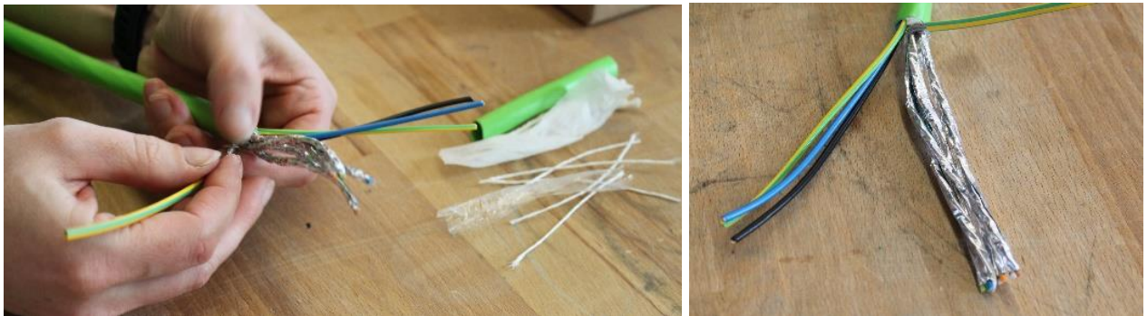
Figure 2.4 – Shrinking tube over twisted shielding braid
