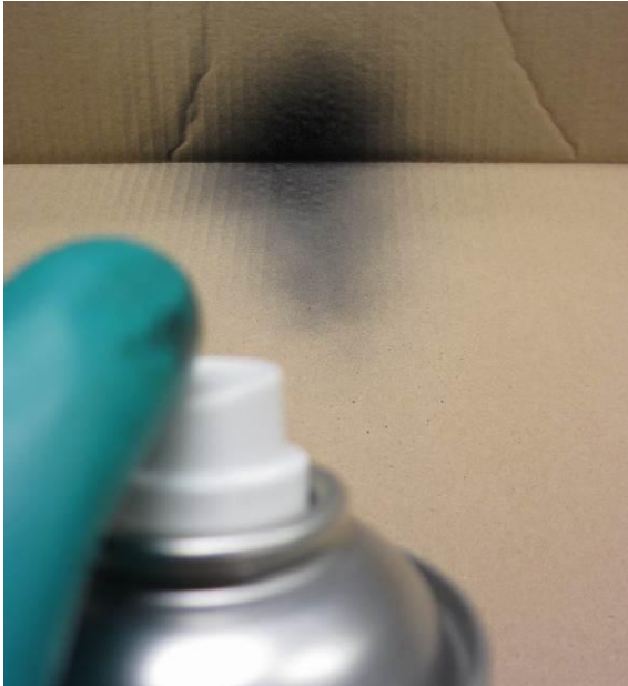
Figure 14, Test nozzle for blockage.
