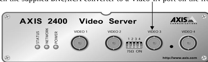
2. Attach the supplied video cable to the converter and plug the other end of the cable into the Video-OUT port of your AXIS EVI-D30/D31 PTZ camera.
