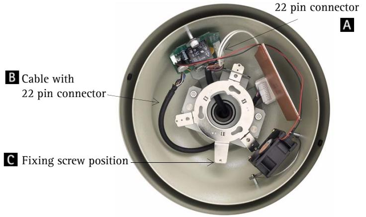
1. Thread the 22 pin connector from the outdoor housing power supply box through the top of the outdoor housing (and mounts) and connect to the 22 pin connector in the outdoor housing **A**.
