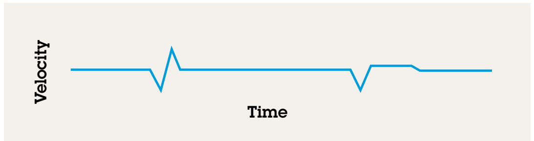
Figure 4. Velocity with irregular disturbances, first symmetric and second asymmetric. Such irregular drops and peaks may be caused by, for example, momentarily increased load or friction. They will always have both positive and negative components.
