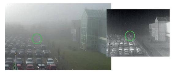
These images compare a 384x288 thermal camera to a 1280x800 visual camera. As you can see, despite the resolution difference, the detection capability of the thermal camera outperforms the visual camera – again.
