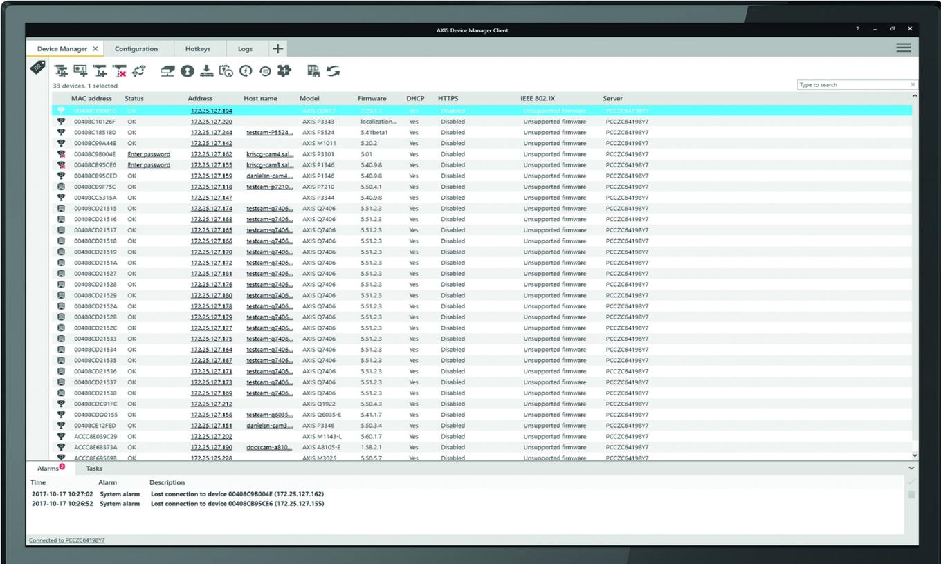
The screenshot displays the AXIS Device Manager interface. At the top, there are tabs for 'Device Manager', 'Configuration', 'Hotkeys', and 'Logs'. Below the tabs is a toolbar with various icons for device management. The main area shows a table of 33 devices. The table has columns for MAC address, Status, Address, Host name, Model, Firmware, DHCP, HTTPS, IEEE 802.1X, and Server. The bottom section shows an 'Alarms' log with columns for Time, Alarm, and Description.
