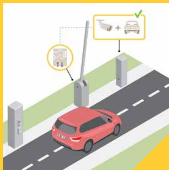
The vehicle entry and exit system offers two options to control the barrier: connect via the camera's internal I/O port or use an external relay module.
