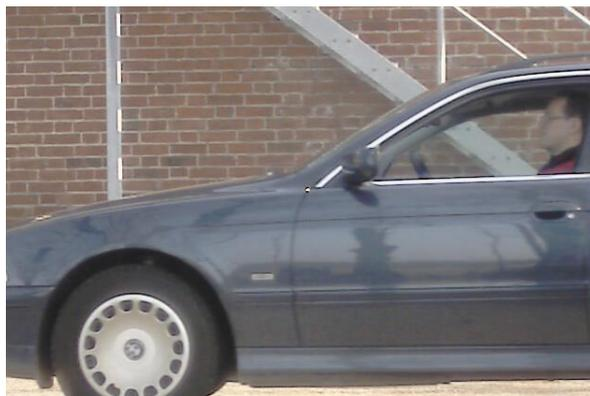
The phenomenon known as interlacing affects analog cameras at high resolution, causing moving objects to blur even when the analog camera is connected to a DVR. Interlacing problems are depicted in the image on the (top). Network cameras that employ progressive scan technology more clearly depict moving objects, as shown in the image on the (bottom).
