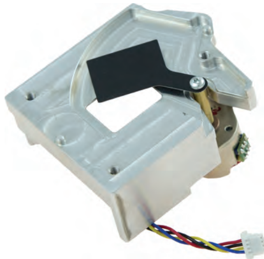
Figure 5.6 A mechanical shutter for a thermal camera. The shutter is used for temperature calibration of the sensor.
