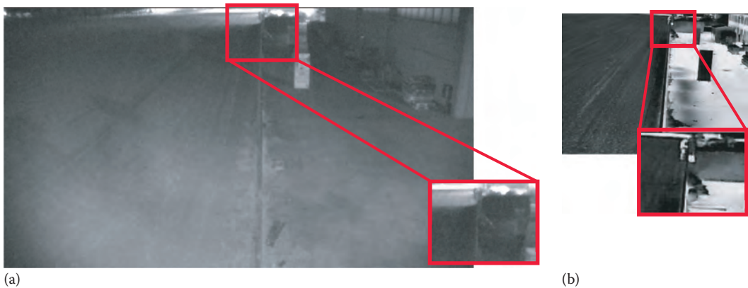
Figure 5.5 Infrared (IR) cameras switch to black-and-white mode to deliver better images in low-light scenes (a). Thermal cameras use differences in heat to provide detection in completely dark scenes and harsh environments (b). Even though the resolution is lower, the thermal camera can detect a person in situations where the IR camera cannot.
