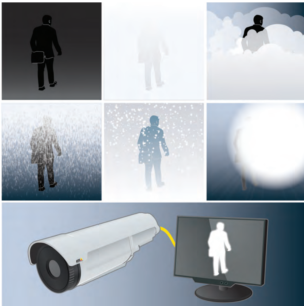
Figure 5.1 Complete darkness, haze, smoke, rain, snow, and even bright and blinding lights—a thermal network camera is still able to detect people and objects.
