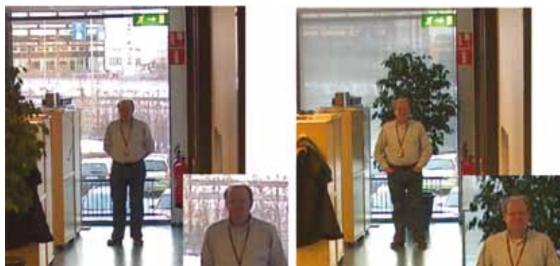
Figure 13. In this scene, blinds and a plant have been used to solve the problem with backlight.
