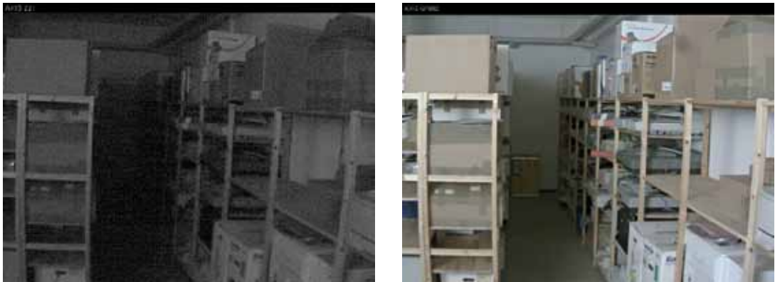
Figure 10. Comparison between a standard network camera and an AXIS Q1602 camera in a low-light scene (0.3 lux).
