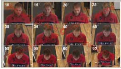
Figure 17. The larger the angle to the object, the more difficult facial features are to recognize.
