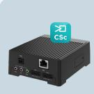
AXIS D3110 with CamScripter App for external USB and IP devices
