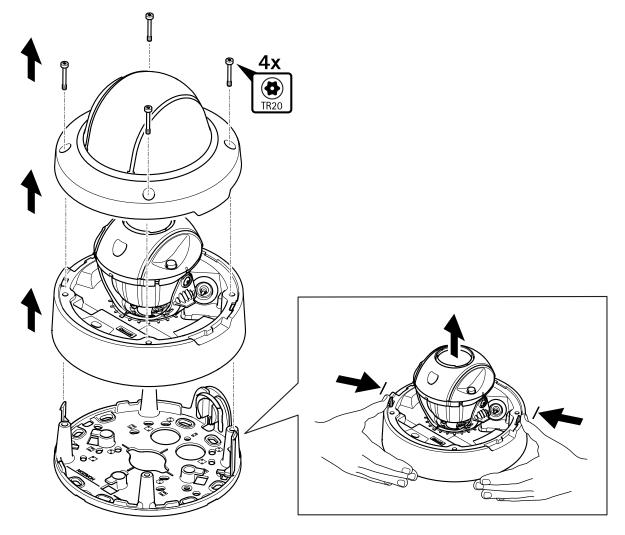
1. Remove the four screws, cover top, holder dome, gasket dome and dome. To remove the mounting bracket, press the plastic clips.
