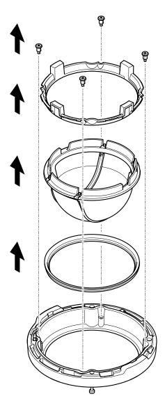
2. Remove the four screws, holder dome, dome and gasket dome.
