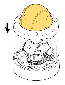
5. Remove the screws from the cover top. Put the cover top back on the camera.
