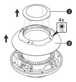
5. Remove the six screws from the ring and remove the ring from the dome.
