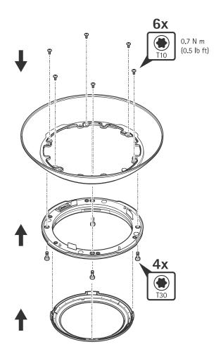
3. Attach the dome assembly to the camera (2 N m).
