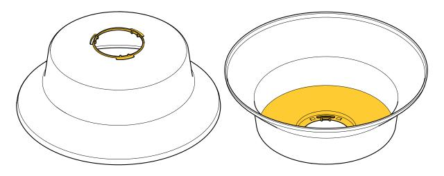
3. Apply a thin and even layer of spray paint according to the instructions of the paint manufacturer.
