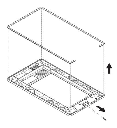
2. Remove the screw (TR10) and the rubber gasket from the inner recess.
