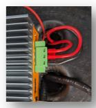
Connect the DIO terminal block to the DIO port and supply 12v dc to pin 1 and ground to pin 2.
