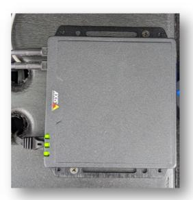
Run the coax cable for the 2 sensors through the vehcile from their install location back to the Axis main unit.
