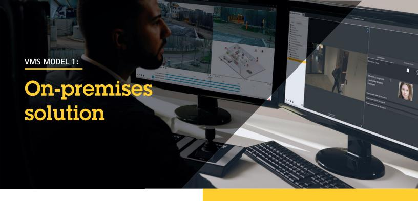
An on-premises video management system (VMS) involves a video server that houses the stored video and is physically located at a customer's site. It requires a climate-controlled environment and usually involves physical devices hardwired and directly connected to a central server.
