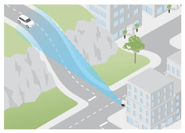
Figure 9. A PTZ camera with sharpdome is ideal in uneven terrain and open areas.
