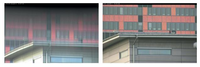
Figure 6. Images from a conventional dome (left) and sharpdome (right) at 20° tilt, 20× zoom.
