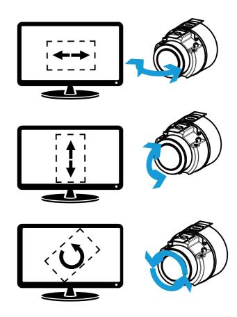
The illustration shows how the directions pan, tilt, and roll affect the live view image.
