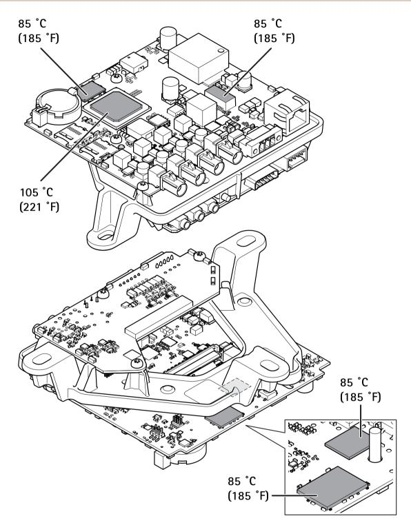
Maximum allowable temperatures. If the ambient temperature is  $35 \degree C (95 \degree F)$  or higher, the temperature of the components increases and they must be cooled.
