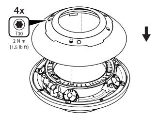
3. Attach the dome assembly to the camera (2 N m).
