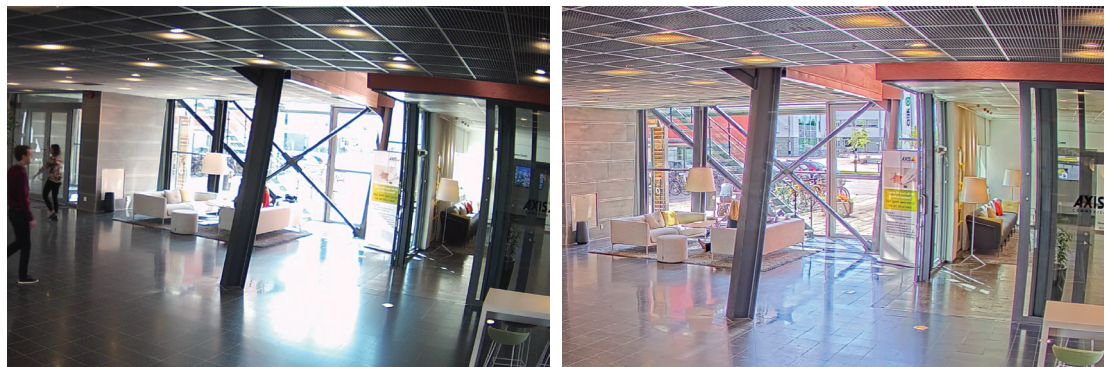
Figure 5 and 6: Indoor scene with strong back-light. Comparison between a conventional network camera without WDR capability (left) and an Axis camera with Forensic WDR (right).
