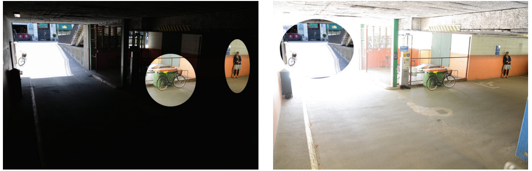
Figure 3 and 4: The same scene as before. The image to the left shows details that were missed with the short exposure time. The image to the right shows the details that were missed with the long exposure time.
