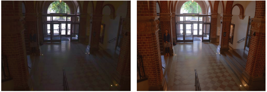
Figure 7 and 8: Back-lit interior captured by cameras with different dB values. The image to the right was taken with a camera with a lower specified dB value than the image to the left, contrary to what could be expected.
