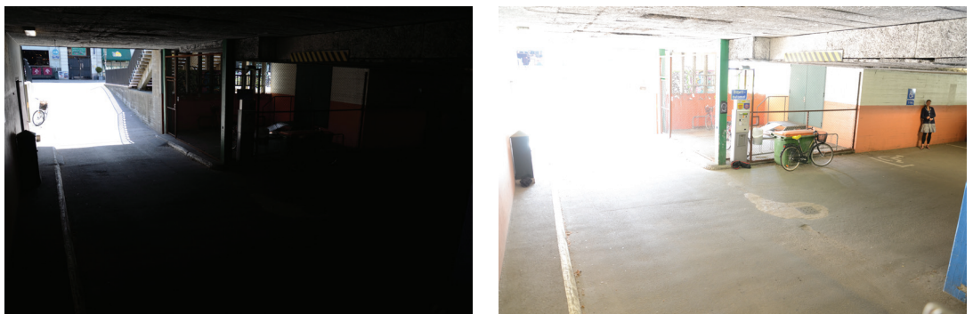
Figure 1 and 2: A typical surveillance scene with a wide dynamic range: a parking garage interior with entrance. The two images were taken using different exposure times, shorter for the image to the left, and longer for the image to the right.
