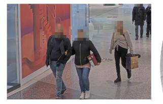
Al-based masking is supported in selected cameras with a deep-learning processing unit (DLPU). With Albased masking, you can analyze live video for human forms, and mask either humans, or the background. This functionality is applicable to near-range indoor and outdoor scenes.
