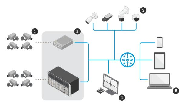
Figure 2. Video encoders (2) provide a solution for integrating analog cameras (1) with a network video system. This consists of network cameras (3), computers with VMS (4), and remote access from laptops or wireless devices (5).
