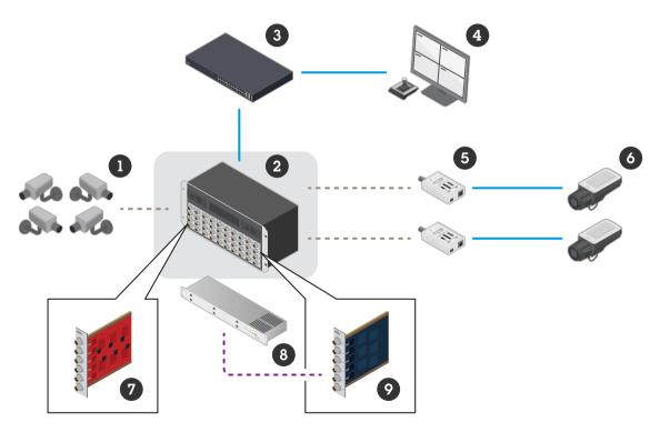
Figure 10. A network video system that utilizes existing coax cables and a video encoder chassis (2). A mix of video encoder blades (7) and Ethernet over coax adapter blades (9, receiving power from a power supply unit, 8)) is used in the chassis. Analog cameras (1), as well as network cameras (6) combined with
