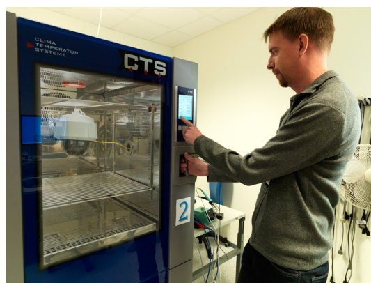
Figure 6. Temperature test in a climate chamber.
